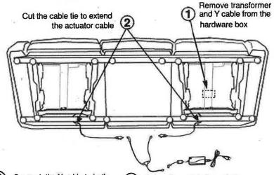
Connect the Y cable to both the actuator extension cable and the transformer.
