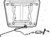
Cut the cable tie to extend the actuator cable
