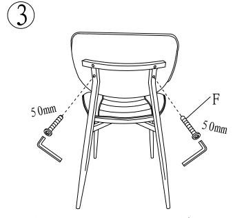
Tighten bottom screws 70%, Then tighten all 100%.
