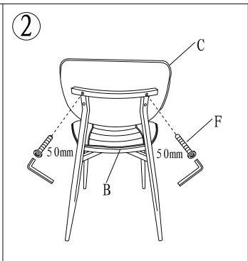
Tighten the screws on the top 70%.
