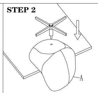
Place the leg into backrest than turn it over and make sure is locked properly
