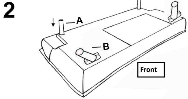
2. The Back Legs Can be twisted into the holes . The front legs will require bolts(E) to be put on with the Hex key(C) on the front. Make sure one washer(D) is put onto each bolt before assembly . Once All four legs are tightened , two or more people are required to flip over the sofa bed and it is ready to be used.
