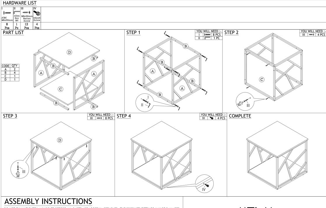
DO NOT FULLY TIGHTEN ANY BOLTS BEFORE ALL PARTS ARE LOOSELY ASSEMBLED. THE PRODUCT/FITTINGS MAY BE DAMAGED IF OVERTIGHTENED. BEWARE OF CROSS THREADING SCREWS AND BOLTS DURINGS ASSEMBLY.
