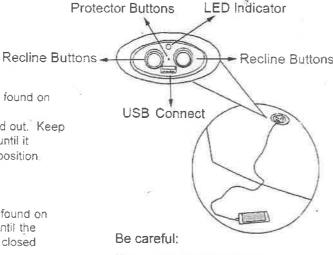
Users may activate/deactivate the protection button by using a pen. Ensure that the protection button is deactivated prior to use. The LED indicator will emit a green light when the power recliner unit is plugged to a power point. The LED indicator will emit a red LED light when the recline buttons are activated.
